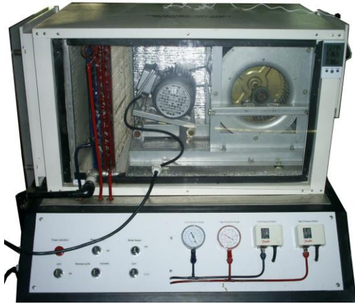
Air Handling Unit
